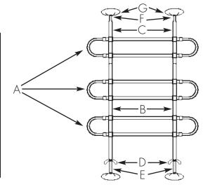
1. Insert Vertical Upright Tubes (B) through the upright support brackets on two of the Telescoping Horizontal Tubes (A).
