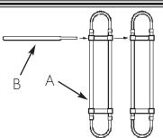
2. Slide the Upright Extension Tubes (C) onto the two tops of the Vertical Upright Tubes (B).
