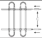
3. Attach the remaining Telescoping Horizontal Tube (A) to the ends of the Vertical Upright Tubes (B).
