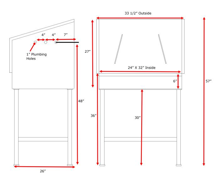
Available as Left, Right or center drain.  $3.5^{\prime\prime}$  drain hole, located  $7^{\prime\prime}$  on center from the left or right.
