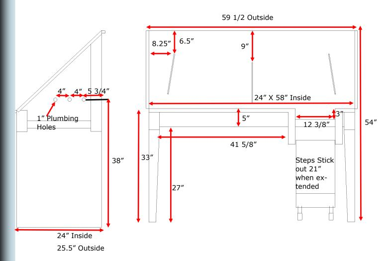
Available as Left or Right drain. 3.5" drain hole, located 7" on center from the left or right.
