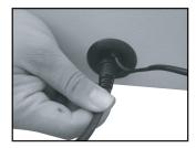
14) Slide the cord from the new electric lift mechanism through the rubber gasket on the electrical control box.
