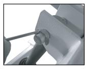
Use a flathead screwdriver (or other pointed tool) to pull out the snap rings from the locking pins on the electric lift mechanism.
