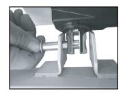
Slide the other locking pin through the mounting brackets at the base of the electric lift mechanism.
