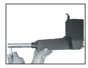
8) Insert one of the locking pins into the attachment hole at the top of the electric lift shaft and rotate counterclockwise to extend, until the tip reaches the mounting brackets on the table/tub frame.
