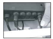
15) Plug the cord from the new electric lift mechanism into the cord port on the electrical control box.
