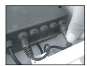
Unplug the cord that connects the electrical control box to the electric lift mechanism.
