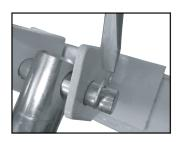
12) Using a flathead screwdriver (or other pointed tool), replace the snap rings to secure the locking pins.
