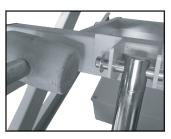
11) Using a hammer, tap both locking pins into place.
