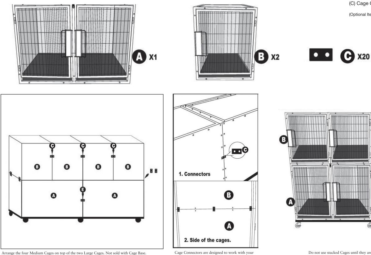
existing cage hardware. Unscrew the bolts at the contact points between two cages. Fit the Connector over the two open holes, then screw in the bolts to secure the Connectors in place. Use at least two Connectors for each touching cage side.
