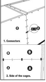
Do not use stacked Cages until they are secured together with Cage Connectors. Shown with optional Small Cage Base (sold separately).
