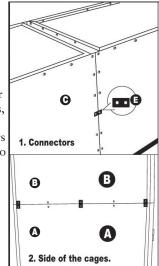
Do not use stacked Cages until they are secured together with Cage Connectors. Shown with optional Large Cage Base (sold separately).
