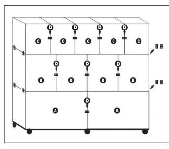
Cage Connectors are designed to work with your existing cage hardware. Unscrew the bolts at the contact points between two cages. Fit the Connector over the two open holes, then screw in the bolts to secure the Connectors in place. Use at least two Connectors for each touching cage side.
